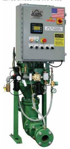
categories, Dilute Phase and Dense Phase conveying. Dilute Phase generally works by vacuum or low pressure air of up to 20 psig and velocities in the pipeline of 4000 FPM and higher, while Dense Phase works by medium pressure air of 10 - 60 psig and pipeline velocities of 2800 - 5000 FPM.
